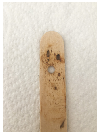
Figure 2: After only a few shots (typically around five to eight) the water content of the wood is greatly reduced by the heat energy, resulting in carbonisation of the wood.
